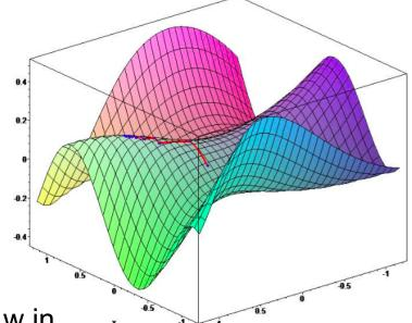
To find a local minimum of J(w), adjust w in direction of the negative gradient:
