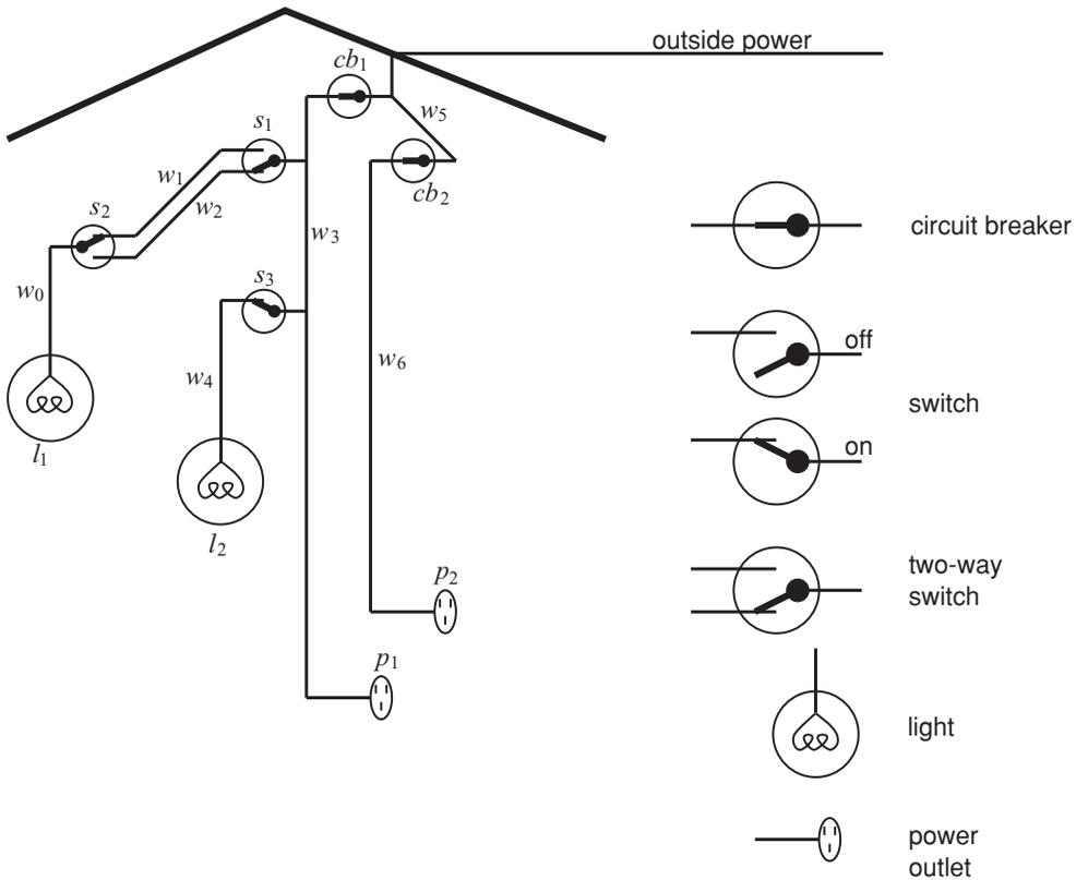
Figure 5.2: An electrical environment with components named
