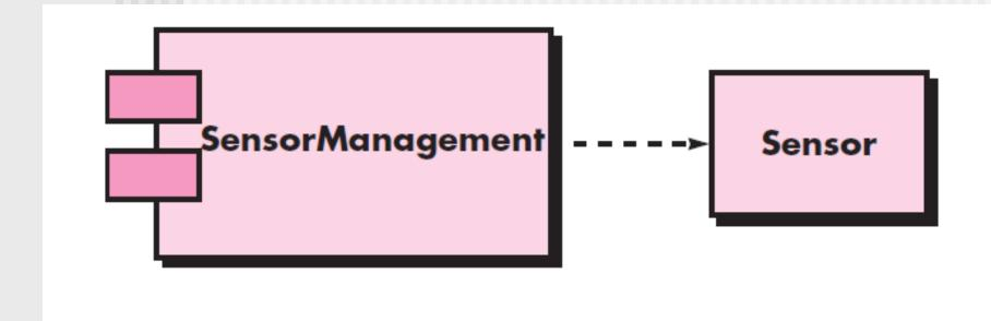
The SensorManagement component performs all functions associated with SafeHome sensors including monitoring and configuring them
