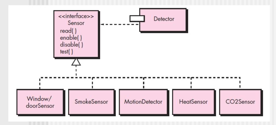
The *sensor* interface presents a consistent view of sensors to the detector component. If a new type of sensor is added no change is required for the **Detector** class (component).
