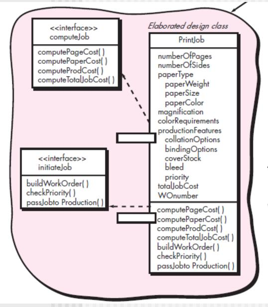
The elaborated design class **PrintJob** contains more detailed attribute information as well as an expanded description of operations required to implement the component.
